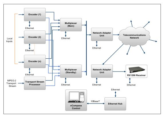
Figure 1.4 Typical Compression System
